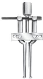
**Internal pulling attachments** have narrow jaws which extend through the center of the part to be pulled. They provide a straight pull and avoid damaging housings. Internal attachments feature adjustable jaws to fit various diameter parts. (Page 129)
